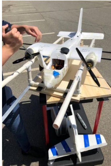
Figure 1. Magnetometer calibration testing on custom turntable.
