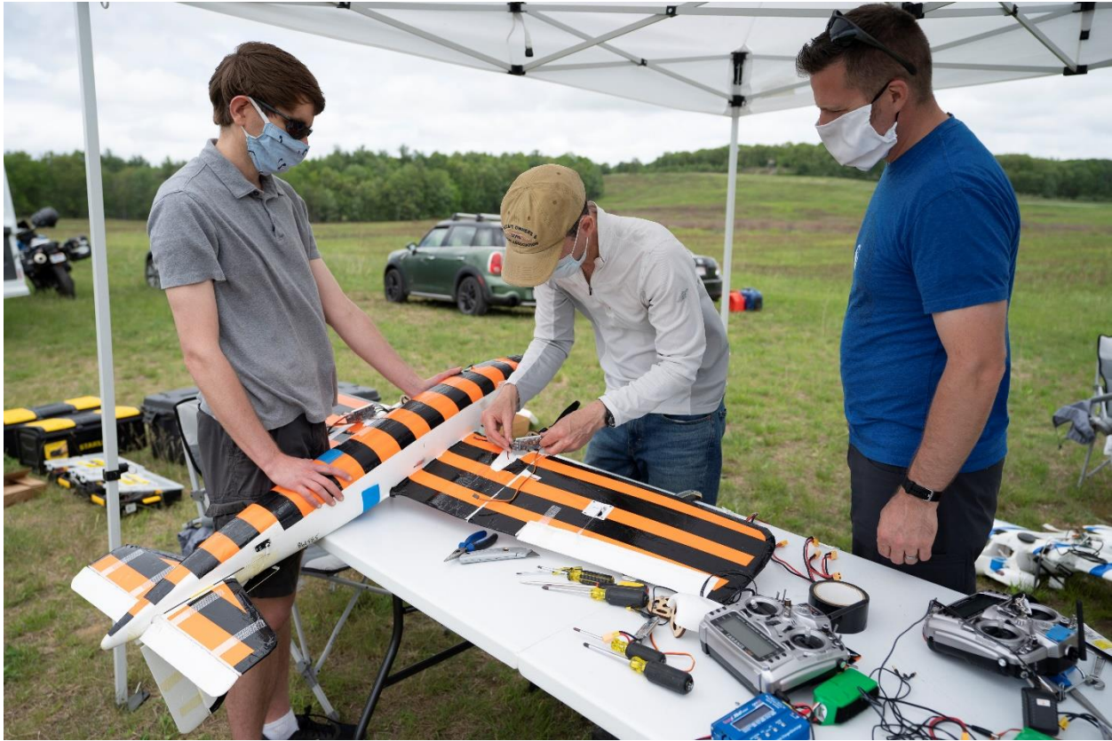
Figure 17. Field replacement of platform motors and power control units. Customized airframe modification was necessary for installation of parts not originally intended for unit.
