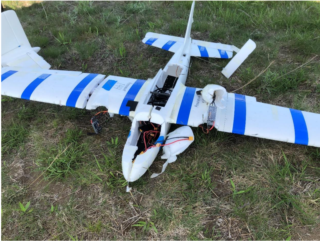
Figure 16. Negative effect of loss of control due to communications failure. Complete separation of motors from wing mounts and cracked fuselage. Creative overnight reconstruction produced a flyable platform.
