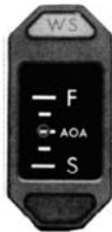
Windshear warning light on PMS speed deviation indicator
