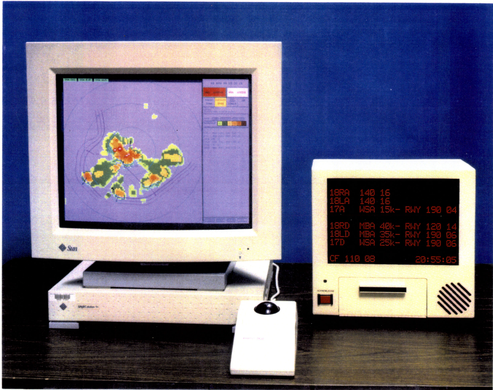
Figure 1. Geographic Situation Display (GSD) (left) and ribbon display terminal (RDT) (right) that convey information on wind shear and other weather phenomena to controllers.
