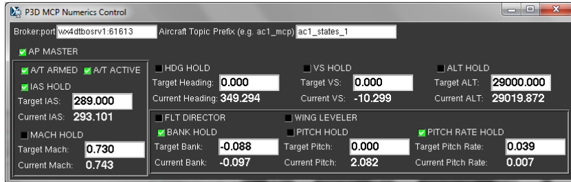
Figure 30. Autopilot Mode Control Panel Interface Providing Target and Actual State Conditions
