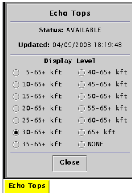
Figure 7-5. Echo Tops product status button and product status dialog box. The yellow button indicates that the product is filtered. In this example, only tops above 30,000 feet are displayed.
