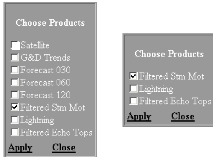
Figure 4-4. Stm Mot product status dialog box and Stm Mot product status button. The yellow button indicates that the Storm Motion product is filtered as a function of window zoom setting.
