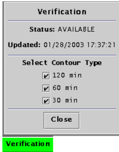
Figure 11-2. Verification dialog box and status button for the Forecast Verification Contours product. The green Verification button and check marks indicate that all (the 120-min, 60-min, and 30-min) of the verification contours are displayed. CIWS Web Site
