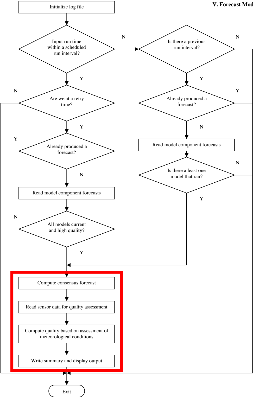
Figure 20. Functional flow diagram for the consensus model, from the Real-Time System and Display Document.
