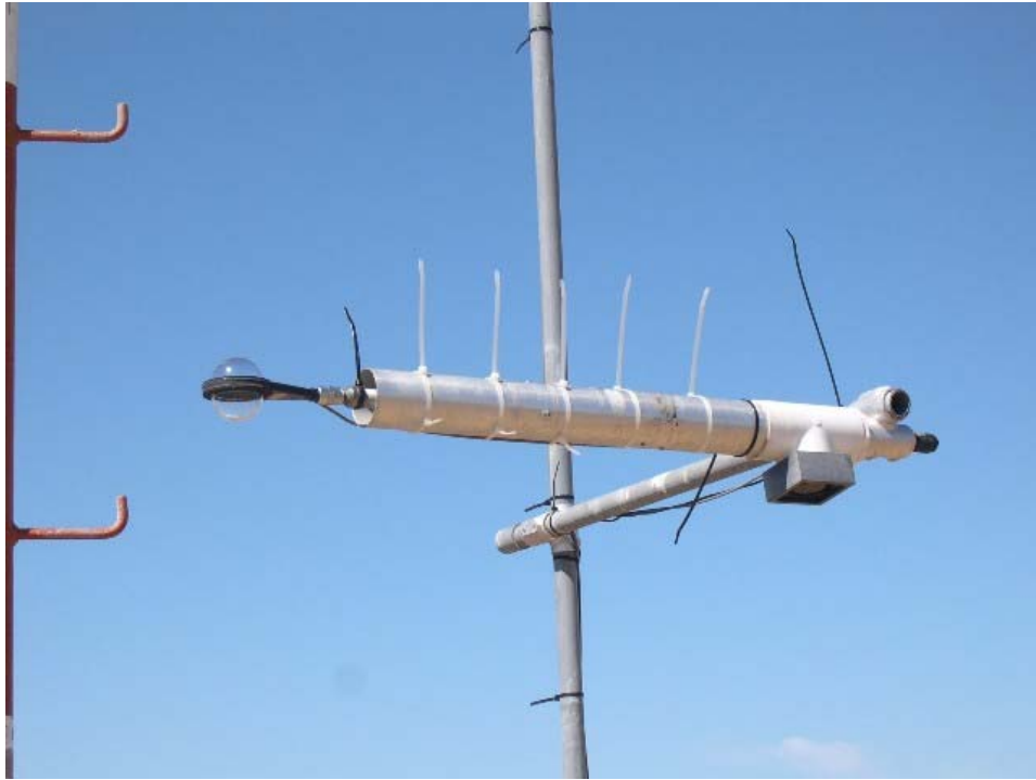
Figure 7. Pyranometer system mounted on lower portion of tower. Sensor is inside glass dome on left.
