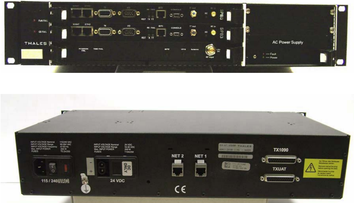
Figure 1. Thales AX680 receiver unit front (top) and back (bottom)
