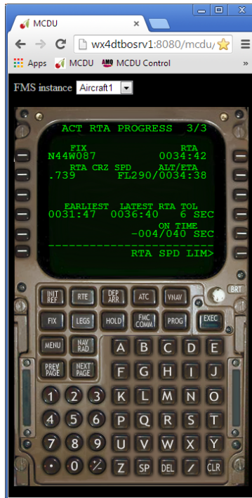
Figure 33. Web-Based MCDU Allowing Observation and Interaction with FMC
